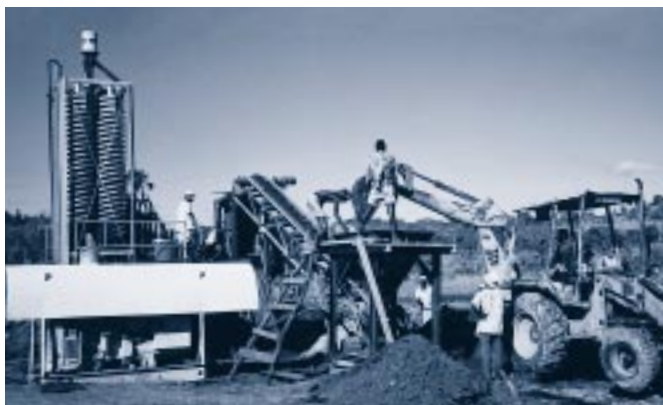
DURING NOVEMBER 1997, THE PILOT PLANT PROCESSED 200 TONNES OF MINERAL SANDS FROM KWALE CENTRAL & SOUTH DUNES.
