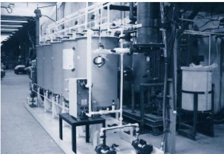
TSR PROCESS: LEACHING CIRCUIT DEVELOPED BY TIOMIN TO PROCESS ILMENITE INTO SYNTHETIC RUTILE.
